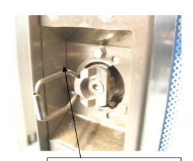
The edge of the centering plate should touch the door.
