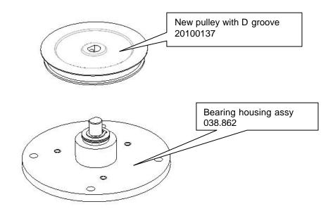
As the pulley now has a D track and the contact face of the driving plate pin has become larger, the new parts cannot be used together with old parts. Consequently, a modification kit, part No 20120200, for older ovens is available.
