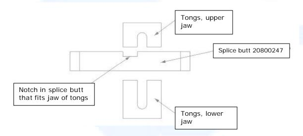
Of course, the splice butts can also replace plug connections on ovens in operation.
