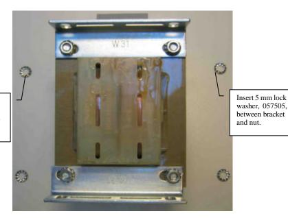
Insert 5 mm lock washer, 057505, between bracket and nut.
